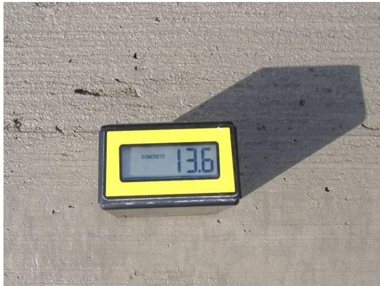
Figure 4.4 James Instrument, Inc. M-60 Aquameter
