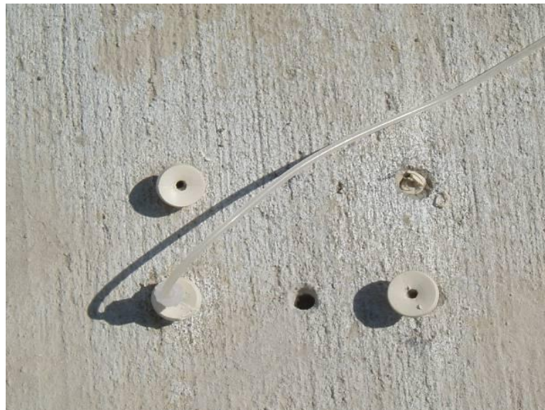
Figure 4.8 Permeability Meter Plug Configuration
