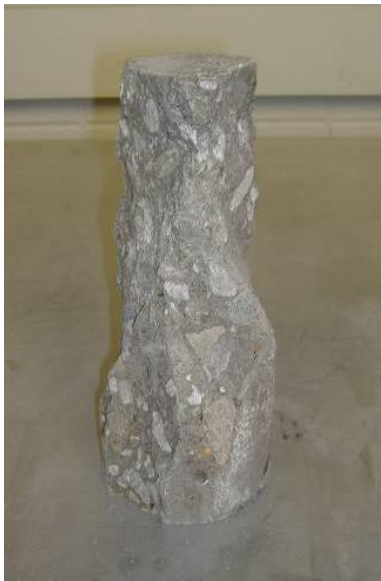
Figure 4.12 Visual Segregation Inspection
